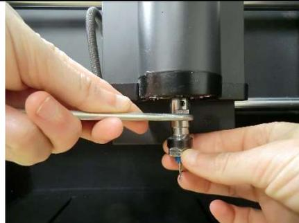
**Step 6: Loosen the nut past its second break-point**
