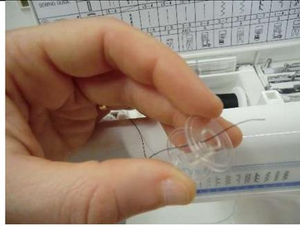
**Step 7: Lock the bobbin onto the spindle**
