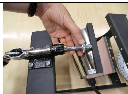
**Step 5: Screw the new attachment into place**
