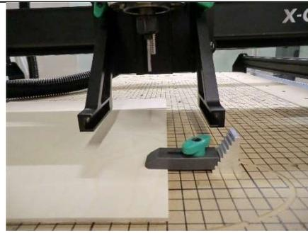
**Step 7: Move the dust shoe rail up until it will clear the clamp**
